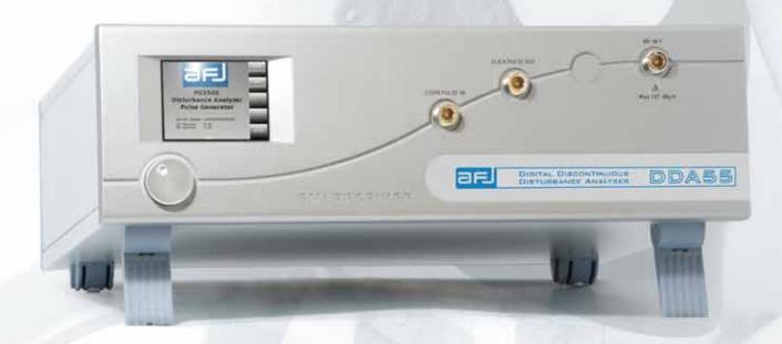
Compact designed and manufactured compliant to CISPR 16 International Standard for measurements of discontinuous disturbances, called "clicks", in accordance with requirements of CISPR 14-1 Standard, advanced software for EMC testing, multi-window real time display, time domain analyse, built-in pulse generator.
