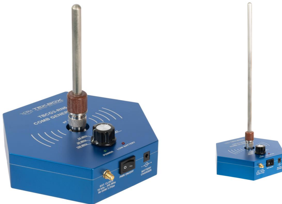
Picture 1: TBCG3-RN6 comb generator
