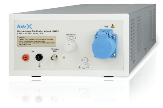
LISN (Artifical Mains Network) is a low-pass filter typically placed between an AC or DC power source and the EUT (Equipment Under Test) to create a known impedance as per complying standard for the measurement of conducted emission. It also isolates the unwanted RF signals from the power source with pre-filter included. It provides a Radio frequency (RF) noise measurement port.
