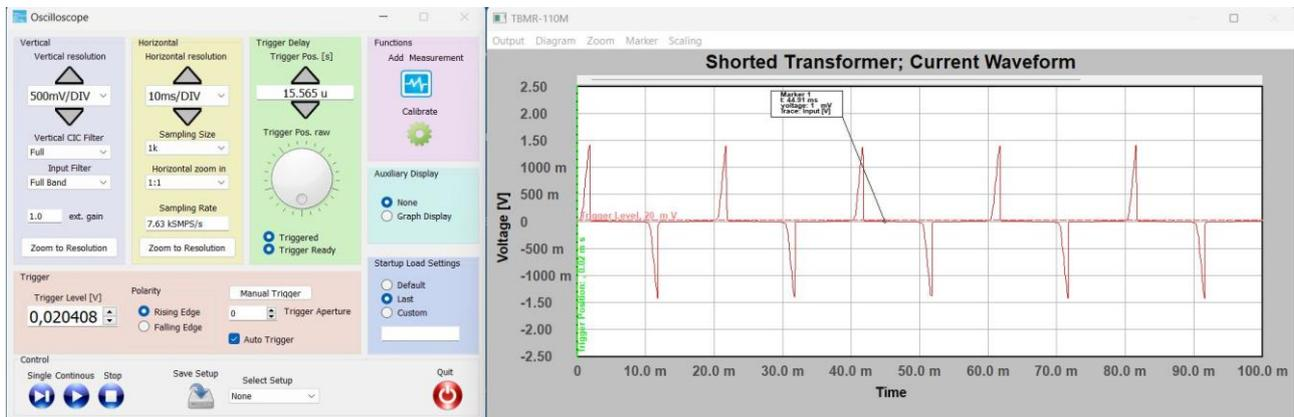
The output current is highly non-linear. This comes as no surprise, after measuring the spectrum.
