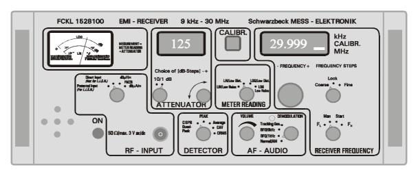
Interference measuring receiver for front panel operation with or without xy-recorder
