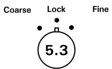
Coarse: 100 Hz - steps in band A 10 kHz - steps in band B Fine: 10 Hz - steps in band A 1 kHz - steps in band B
