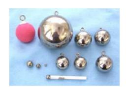
The ED&D Impact Test Balls are high-precision machined steel balls, usually chrome plated, used to test impact resistance according to IEC, CSA, CE, EN, MIL, VDE and UL Standards...among others. The units come with removable eyelets, where applicable. The balls come with ISO/IEC 17025 Accredited, in Scope, calibration. NIST-traceable.
